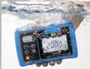
IP67 protection, even with the terminal caps open
