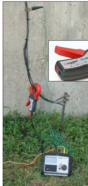
Current measuring clamp (inset) for ART testing capability
