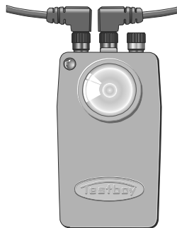
Continuity test with buzzer
